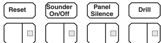
Pressing **Sounder On/Off** turns off all sounder circuits defined as audible. The yellow LED turns on when silence is activated via the Sounder On/Off or via the alarm silence software timers.
